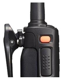
Man-down Detection, Stationary Detection, or Motion Detection will be automatically engaged when the embedded acceleration and tilt sensors detect unusual behavior. Lone Worker function automatically places the radio in Emergency Mode if it is not operated for a certain period of time. The bright orange Emergency Button is located at the top (portables) or front (mobiles) of the radio for high visibility and instant access when needed.
